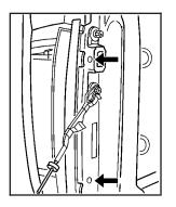
Remove the two rear lamp assembly screws near the tailgate latch.
